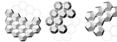
Three types of topological interlocking of dodecahedra, TI 1, TI 2, TI 3. (© Vera Viana)
